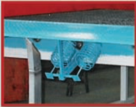
THE OPTIONAL EDGE-OF-DOCK FEATURE bridges the transition from the ramp into the truck. A mechanical torsion spring lift assist allows operation by one person. The bridge permits access to trucks 3" - 4" higher or lower than the ramp and comes complete with bumper blocks.
